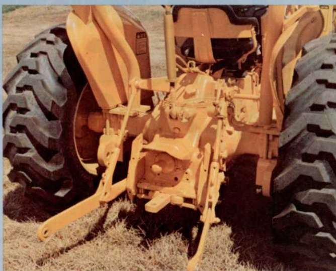
Leveling 3-point-mounted tools is easy using the hand cranks located on the lift link and right draft link.
