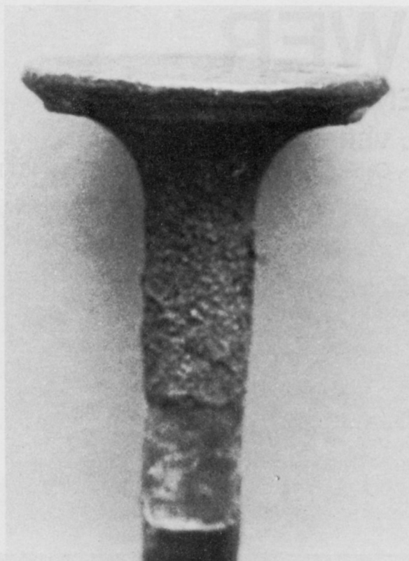
Valve stem erosion (top) indicates the fuel mixture is too lean or condensation inside the engine. Damage to entire circumference of the valve face (bottom) is caused by insufficient valve clearance.
