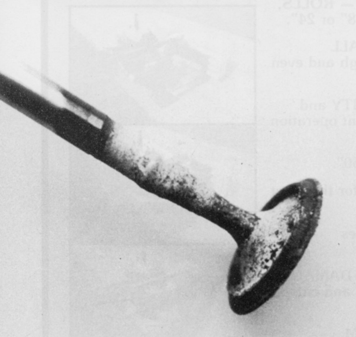
Valve stem erosion (top) indicates the fuel mixture is too lean or condensation inside the engine. Damage to entire circumference of the valve face (bottom) is caused by insufficient valve clearance.
