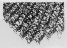
Enkamat, available from Turfibre Products, is a three-dimensional turf fibre mat to strengthen and stabilize turfgrass areas. It is made of strong, surgical quality nylon threads, fused together into an open three-dimensional web matting. Ninetenths of its volume is open space. Environmentally safe, Enkamat is unaffected by humic acids or soil fungi.
