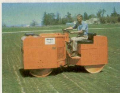
A six-ton roller was used in this case to smooth the surface. This would not be possible with a soil field.
