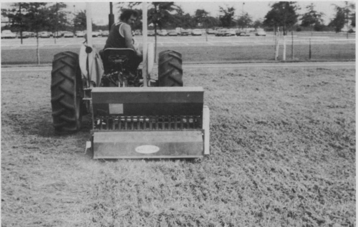
An Aeroblade and cross-seeding were used prior to seeding to help obtain a faster knit.
