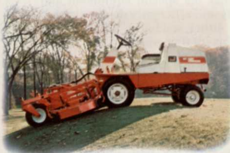
Cutter deck tilts up and down for mowing gullies and bank edges.
