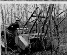
Easily handles dense brush, 6" dia. trees in a single pass; reduces material to mulch — discharges downward; eliminates burning, hauling; provides immediate access to cleared area.
