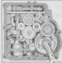
Gravelly's all-gear direct drive. A transmission with a lot of teeth in it.
