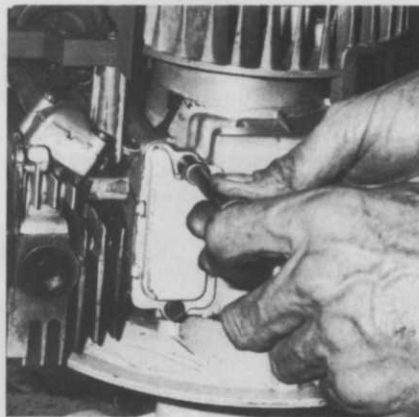
Remove the cover over the valve springs.
