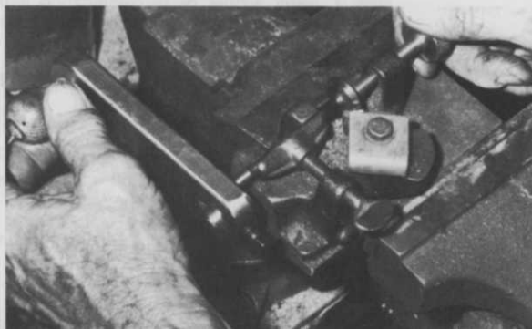
Place it in the refacing tool and tighten the bolt shown on the right until the valve face is against the cutting unit. Turn the handle while tightening the bolt until the valve face is even.
