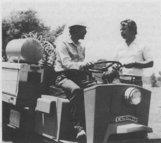
Superintendent Richard Eicher instructs operator of irrigation service vehicle at Lakeside Country Club in North Hollywood, Calif. A Cushman flat bed cart has been equipped with service box, sprinkler rack, pipe vise and air tank.
