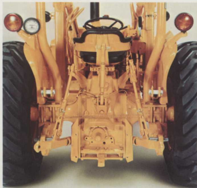
Draft links can be one-piece or telescoping. They are easily adjusted and the leveling crank can be locked.
