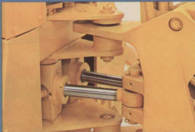
The 9250-A Backhoe utilizes dual swing cylinders that provide 11,083 foot-pounds of swing torque.
