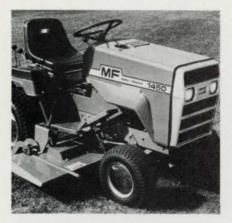
Massey-Ferguson introduces the new-from-the-grass up MF 1450 and MF 1650 tractors. Both are designed for a wide variety of lawn care jobs. A 650 lb. capacity, 3-point hitch and rear PTO are available as options. At 14 and 16 hp, they come with hydraulic implement lift and front belt-driven implement device.
