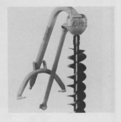
Five Star Engineering has developed a heavy-duty industrial auger digger. The Five Star Digger is sold under a three year warranty and fits all tractors with Cat. 1 & 11 3-pt. hitches. Bevel gear is machined and hardened and Woodruff keyed to the output shaft with a reduction of 3.18 to 1. Pinion is one piece with splined input shaft, machined, hardened and straddle mounted between two tapered roller bearings.
