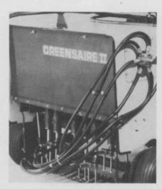
A new liquid injector attachment capable of injecting nematicides up to three inches deep through small, hollow tines, will be introduced this spring by Ryan. The new attachment is powered by Ryan's Greensaire 11 aerator and connects to any pressurized (150-400 psi) spray tank. The attachment can be installed in approximately 30 minutes. The new attachment can treat up to 8,000 sq. ft. per hour.
