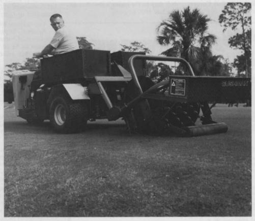
The amazing new Cushman Greensaver ® attachment provides penetration down to 2-1/2", yet gets aeration and cleanup done up to 10 times faster than most methods.
