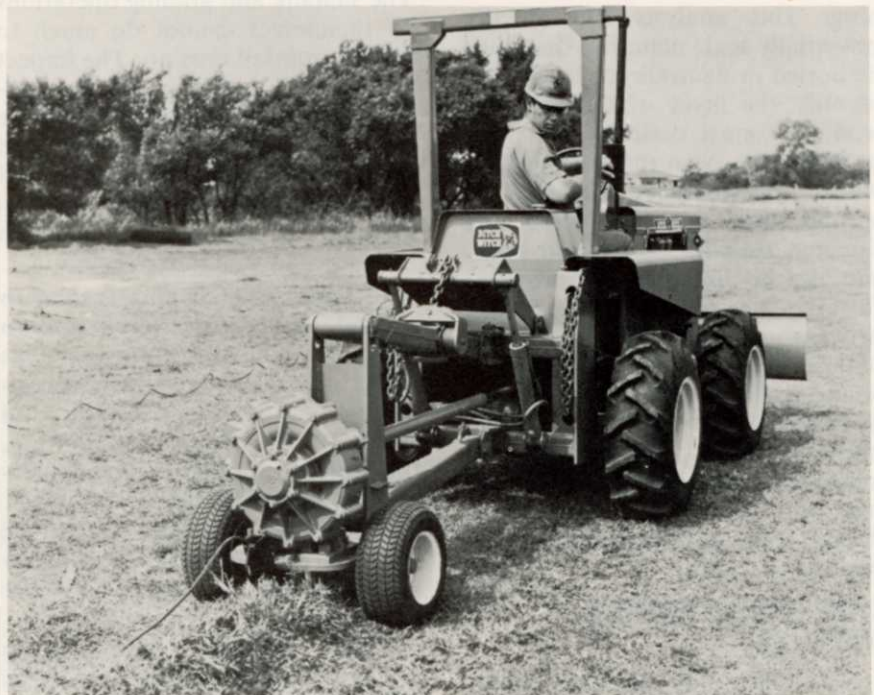
Vibratory plow modules are available for Modularmatic vehicles in the 30-HP to 65-HP range.
