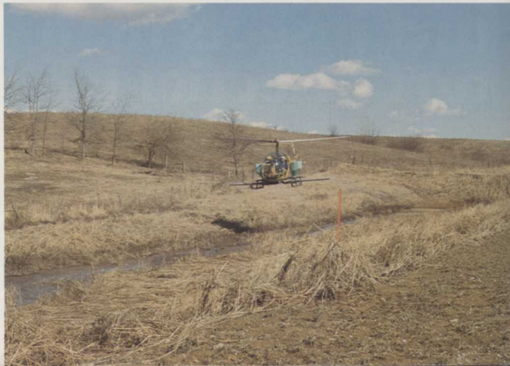
Above: special aerial bucket carries enough seed for eight acres. Right: an altitude of 45 feet with a speed of 45 miles per hour yields a swath width of 45 feet.
