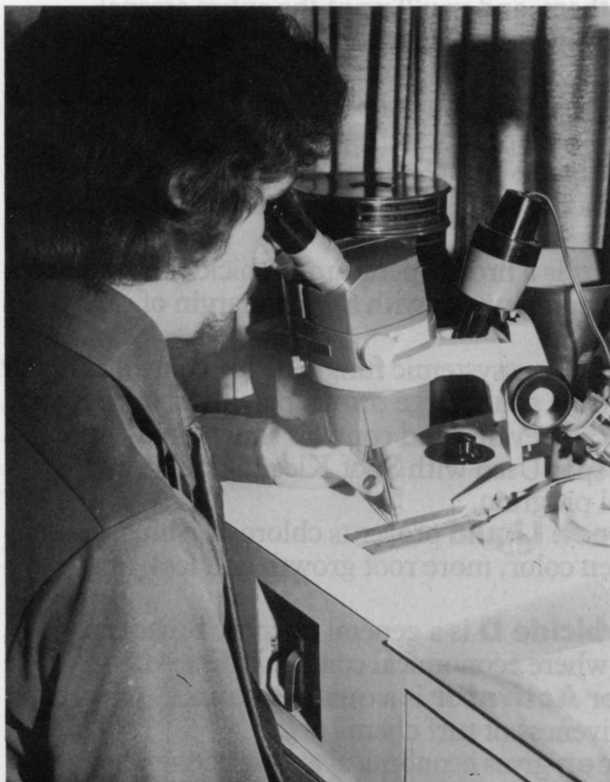
Kevin Kern, technician, uses vibrator developed by Seed Technology, Inc., to check turfgrass seed sample. Vibrator directs seed past operator at a variable speed rate depending on type and condition of seed. Magnification range is 1 1/2 to 25 power. Unit permits careful examination of seed at a rate 10 times faster than hand method, which also includes use of a hand lens.
