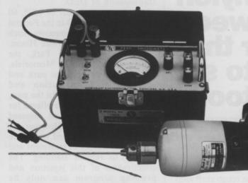
A practical, low cost instrument that pinpoints discoloration and decay in their early stages before they are evident externally. Allows time for early treatment or removal before damage to surrounding area. Ideal for utility pole, park, and recreation area maintenance, and forestry research and inspection.
