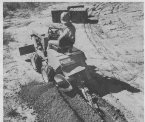
18-HP Model J20 — 4 wheel drive, with three speed forward plus reverse transmission
