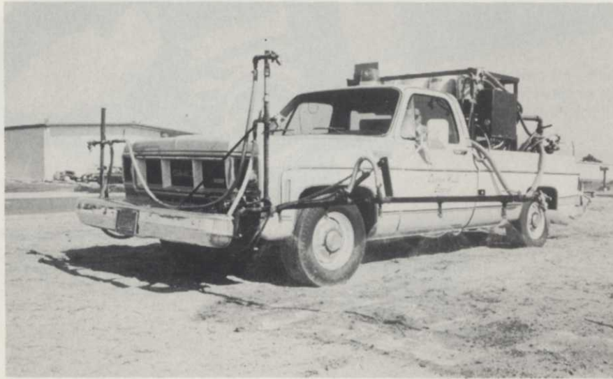
Heffernan has his 3/4-ton pick-up rig equipped with a 320-gallon fiberglass tank, drift-control nozzles with remote controls, a brush nozzle attachment giving him a 35-foot swath with hydraulically controlled booms mounted on the front.
