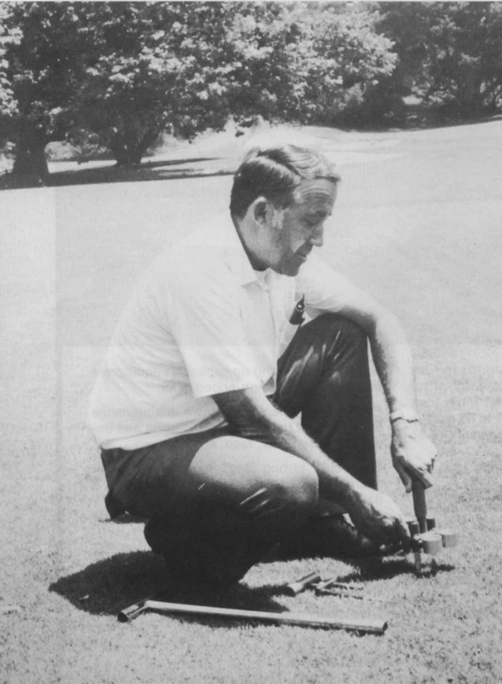
Valley Club superintendent Don Lokey testing moisture level with a moisture sensing instrument to determine water required for the next irrigation cycle.
