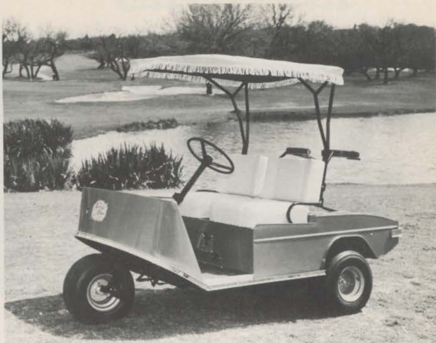
ELECTRIC CADDY from Electric Carrier Corp. has a body made of zinc-grip coated steel and is powered by a traction motor, 36-volt DC.
