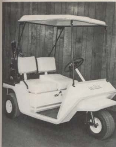
THE MELEX model 102 is an electric car weighing 670 pounds without batteries. It features an automatic seat brake, automotive steering and reverse warning buzzer.
