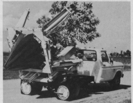
TS-44T—An extremely popular model with extra advantage of single unit mobility. Digs 4 in. diameter trees. Features optional spade extension for handling deep tap roots.
