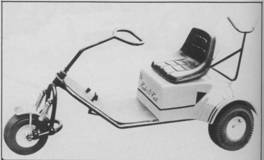
KUSH-N-KART weighs only 283 pounds, and is an electric 3-wheel cart with a spring suspension design. It's made by a firm in Barberton, Ohio.
