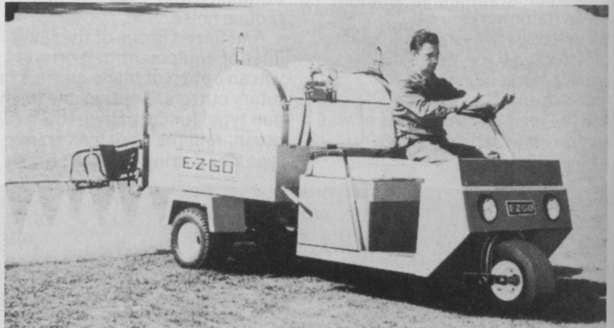
THIS IS the GT-7 Truck from E-Z-GO, re-introduced this year. It's powered by a 20 hp ONAN and has a rated payload of 1,500 pounds.
