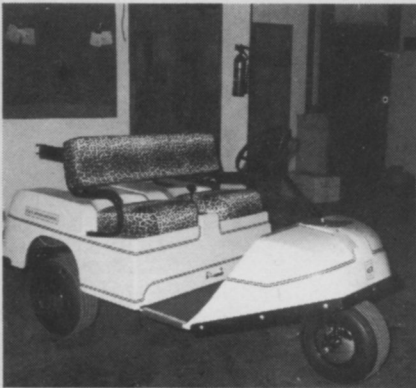
MINNESOTA-based American Continental makes both gas and electric three-wheel golf cars. Length for both models is 91 inches, while the width is 47½. Construction: fiberglass body and steel frame.
