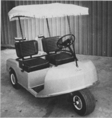
CAPRI-100, from Southern Golf Equipment in North Carolina, is an electric car with rear body latch and cushioned brake to prevent turf damage.
