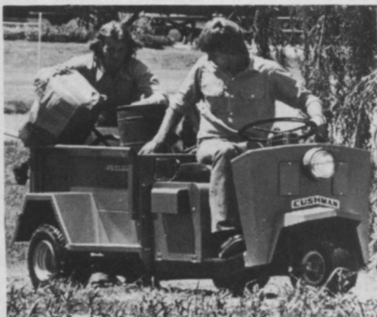
RUNABOUT from Cushman has automotive steering, rear shock absorbers and an 18-hp air-cooled engine.
