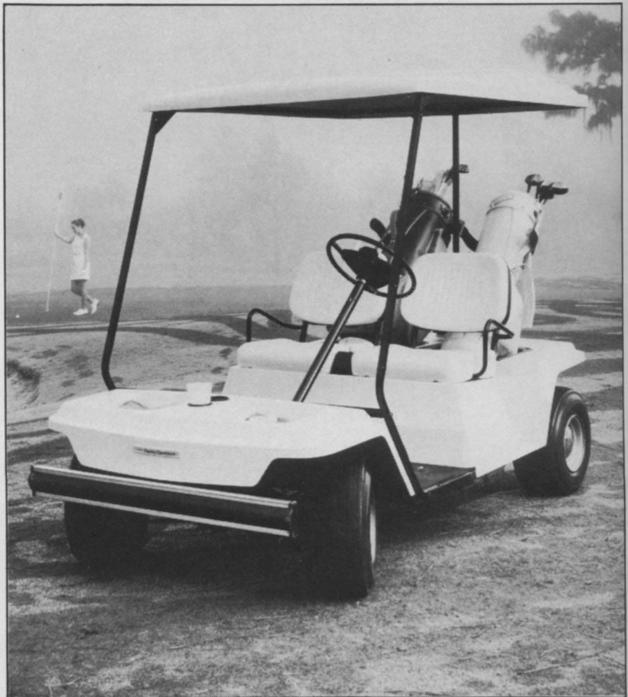
AMF Harley-Davidson's new DE-40, the firm says, can handle a 750-lb. payload at speeds up to 11 mph. An added feature are front beverage wells.
