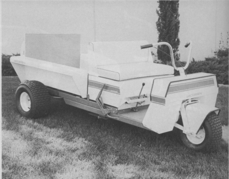
PEOPLE OR TOOLS, up to a 1,000-pound capacity can be transported in this Jacobsen Cruiser 2 truck. It's powered by a 8 HP engine and can move 12½ mph.
