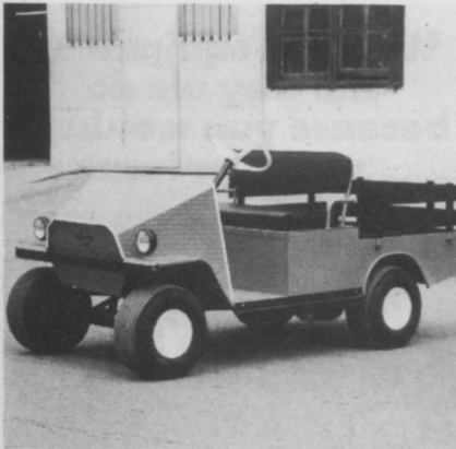
PANTHER, a personnel/burden vehicle from Electric Carrier Corp., is an electric vehicle with a 44" x 36" cargo space. It has automotive steering, disc brakes, automatic parking brake and can be equipped with extra-wide flotation tires.
