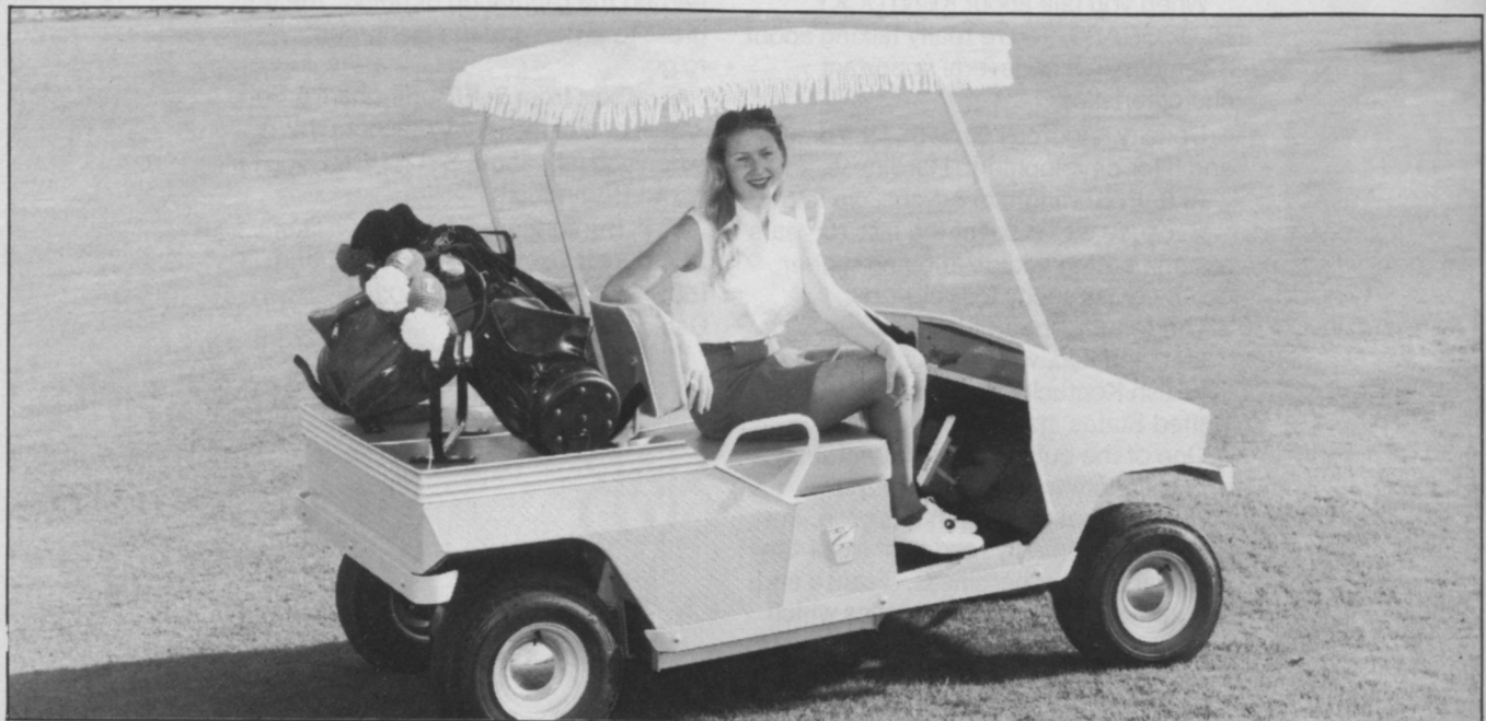
TAYLOR-DUNN's electric car is all steel and features an automotive drive axle and leaf spring suspension. It weighs 1,065 pounds with battery.
