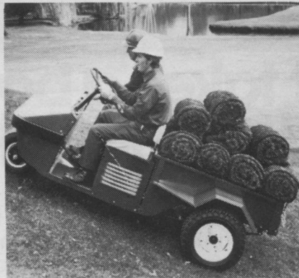
WORKMASTER from Toro has a closed, self-lubricating drive system. It has a 1,000-lb. payload.
