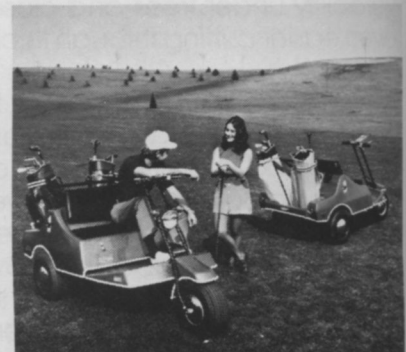
THIS IS the Brute-Car from Lake Sports, weighing only 340 pounds with fuel. It has a fiberglass body, steel frame and is 88 inches long.
