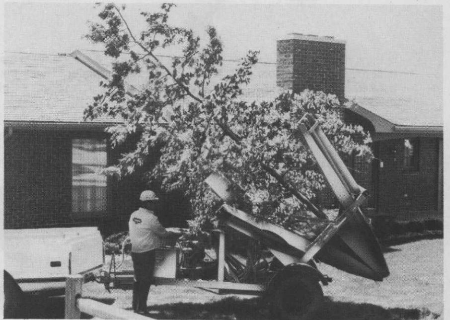
Tree spades also come in completely self-contained, trailer mounted units with their own hydraulic system and power plant. But the shorter over-all length of truck-mounted models make street tree planting easier.
