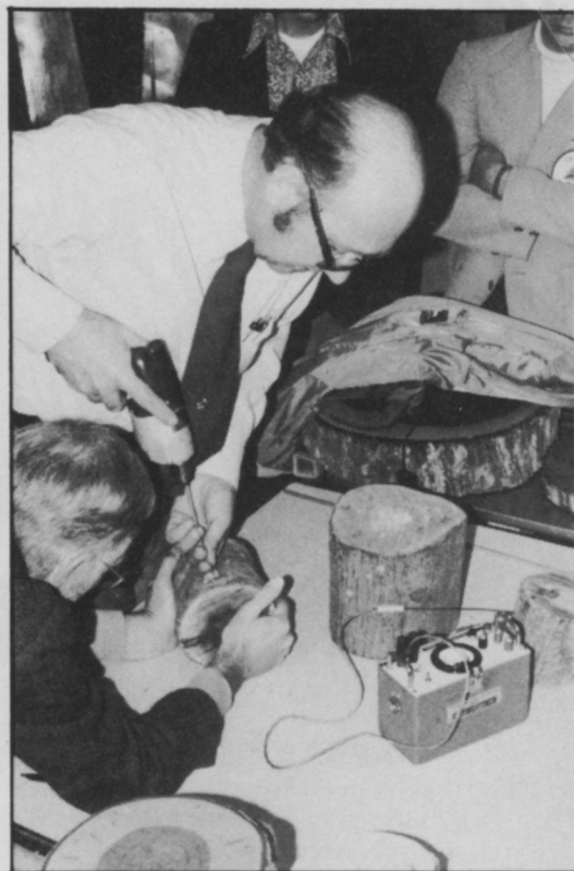
Ed Hogarth steadies a tree section as Alex Shigo drills a small hole in preparation for a demonstration of the "Shigometer," an electrical probe that can measure the advance of decay in a living tree.
