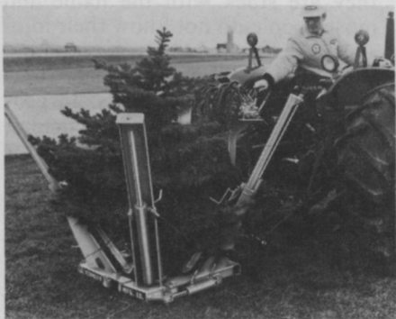
TS-20—Vermeer mini-spade may be mounted in minutes to your tractor's 3-point hitch. Ideal for moving small trees, bushes. Maximum ball size: 20 in. diameter, 18 in. deep.
