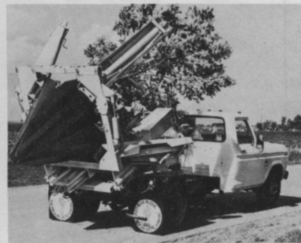
TS-44T—An extremely popular model with extra advantage of single unit mobility. Digs 4 in. diameter trees. Features optional spade extension for handling deep tap roots.
