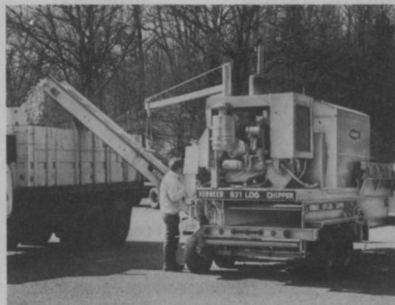
Here's instant log disposal. Vermeer 671 Log Chipper takes lumber, railroad ties, telephone poles and chews 'em to chips in minutes. All hydraulically operated.
