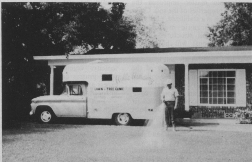
This ten-year-old fiberglass prototype tank mounted on a one ton truck is the result of many years of dreams, ideas and planning.
