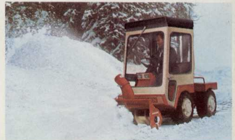
Snow Thrower clears a 48" path directing snow to left or right. Cab is optional.
