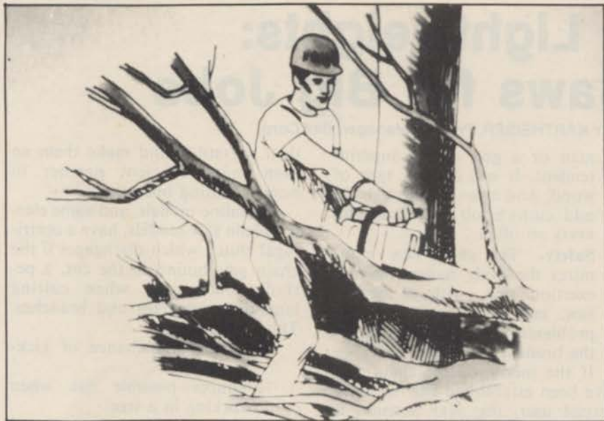
Important factors in operating a chain saw safely are good footing and a clear area.
