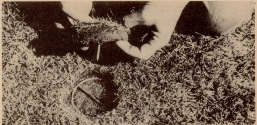
These sod plugs are transplanted and allowed to root. The rooted plugs are used to determine the force necessary to lift the plugs from the soil. The ring with the cross bar is placed under the plug and a nail is inserted so the cross bar can be located later for lifting.
