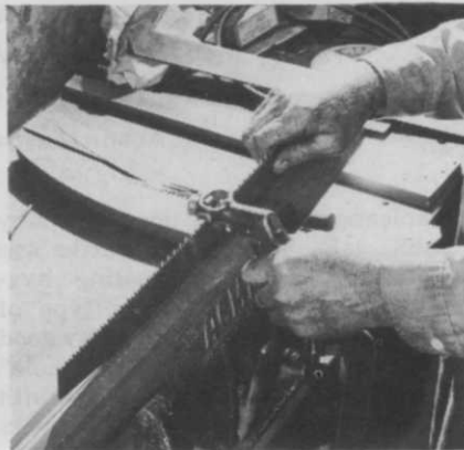
You can buy a pistol-grip saw setting tool for your saws. Stanley Tools makes an acceptable unit. Set the teeth on one side first and turn saw over.
