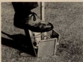
1 Damaged section of turf neatly cut by blades . . . one at a time.
