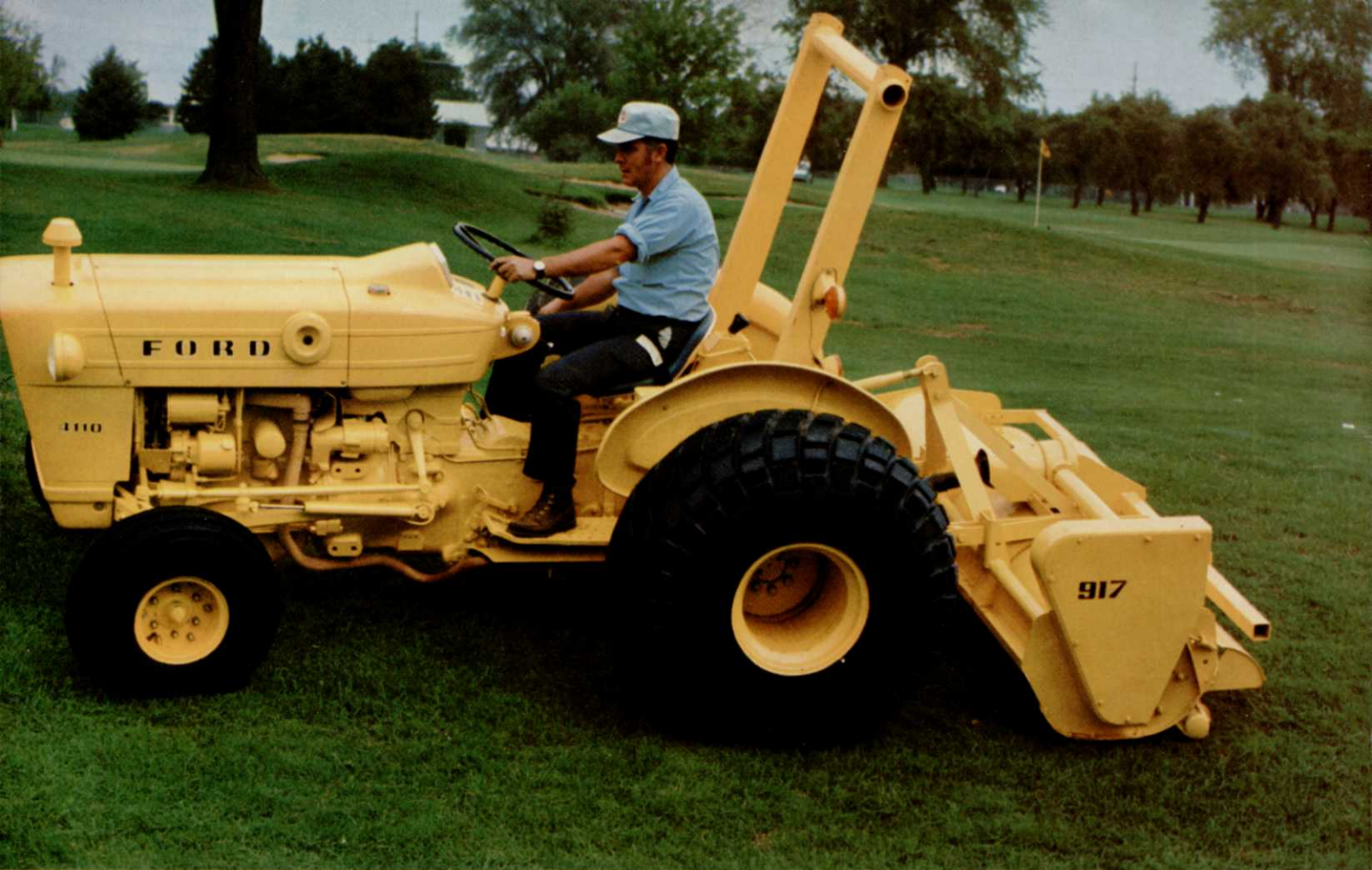
Ford 4110 LCG shown with new 917 Flail mower.
