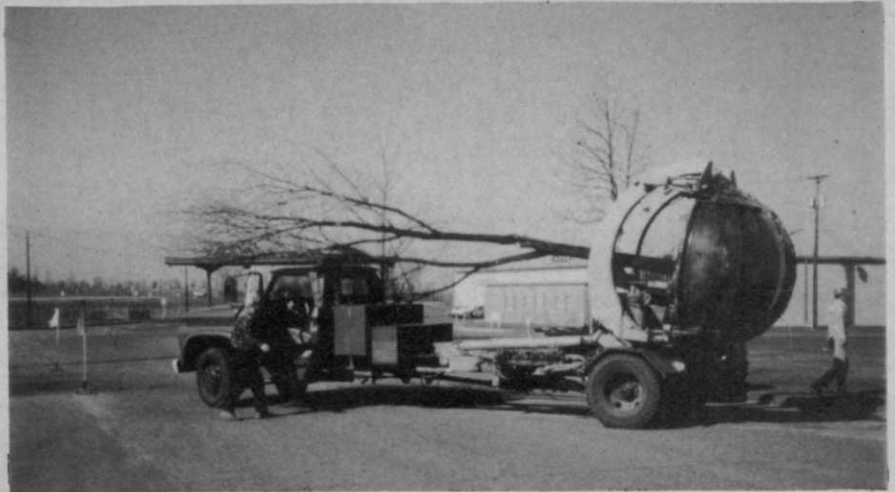
This clam-type digger (72 inch) was developed in 1964 for large tree moving. Authors used clam- and spade-diggers in moving trees.
