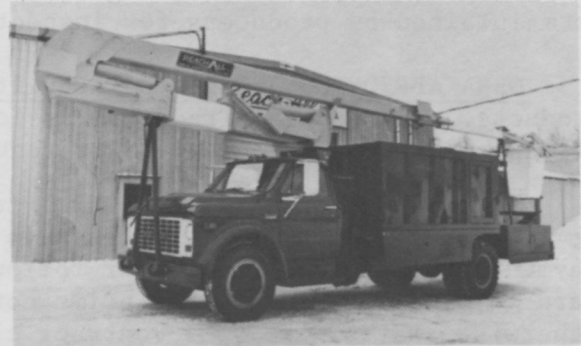
REACH-ALL Model 5050 3K aerial basket with hydraulically powered 12" chipper, a hydraulic ejection box and tool boxes. All assembled as one complete unit.
