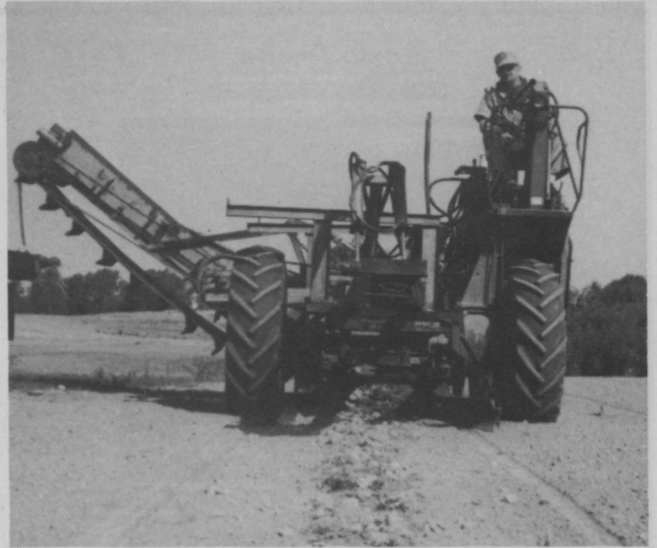
Here's a stone's eye view. Windrowed stones are picked up easily with this converted potato digger-stone picker. Bergman designed and built the picker himself.
