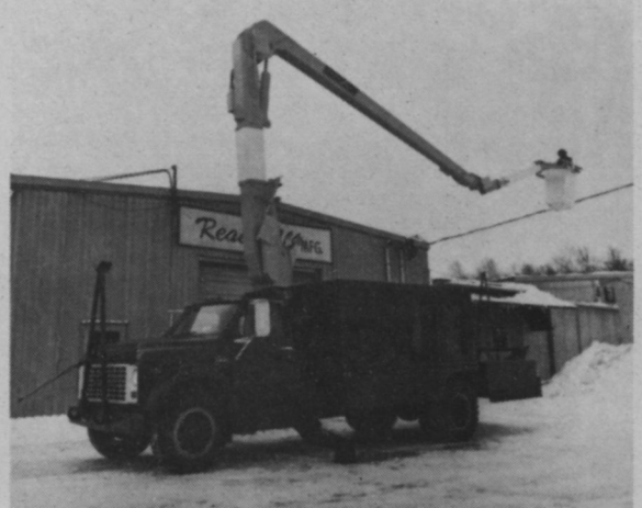
REACH-ALL increases your working area with its modern 3 knuckle design and includes fiberglass lower boom insert.
