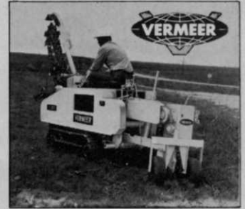
T-218—18 hp buries cable down to 18"
