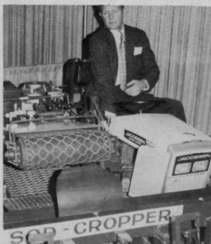
Robert Gieringer, Gieringer Mfg. Co., Milwaukee, Wisc. demonstrates the ease of handling of the Sod-Cropper, a machine used to roll sod.
