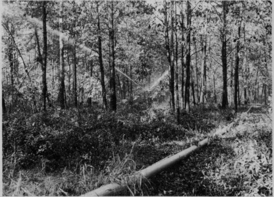
One of several hundred spray nozzles that shoot effluent from the lagoon system into the air over 50 acres of woodland. The trees thrive on it.
