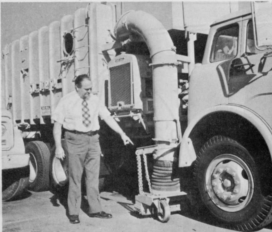
This sweeper was specially designed by Smith and his crews. He points out a leaf attachment which aids in leaf pickup. Large machines such as this receive thorough maintenance at regular intervals.
