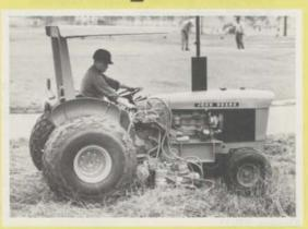
Warm weather? With John Deere, the fuel tank and battery are both mounted well away from engine heat. Cooling system is pressurized with pump, thermostat, and fixed bypass. Air cleaner is dual-stage dry type, sized right for engine capacity.
