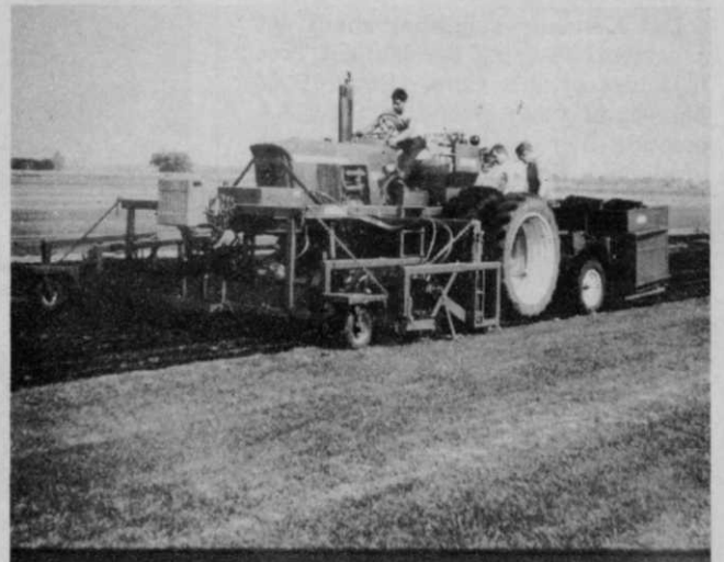
Sod harvester follows closely behind the sod cutter. Conveyor carries rolled sod to four men on rear of machine.
