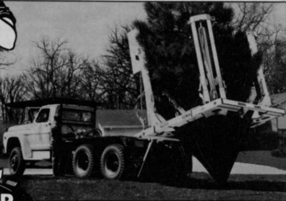
Truck-mounted TS-66T Tree Spade—A high production unit with the extra advantage of single unit mobility. Digs tree ball 66" in diameter, 48" deep. Requires absolutely no hand labor. Hydraulic controls position its high tensile steel spades.
