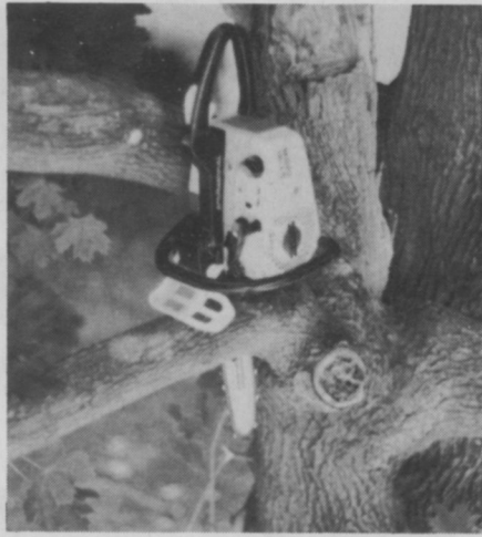
Foolishly hanging saw temporarily on stubs or crotches not only could smash your saw, but also could kill or injure workers below.
