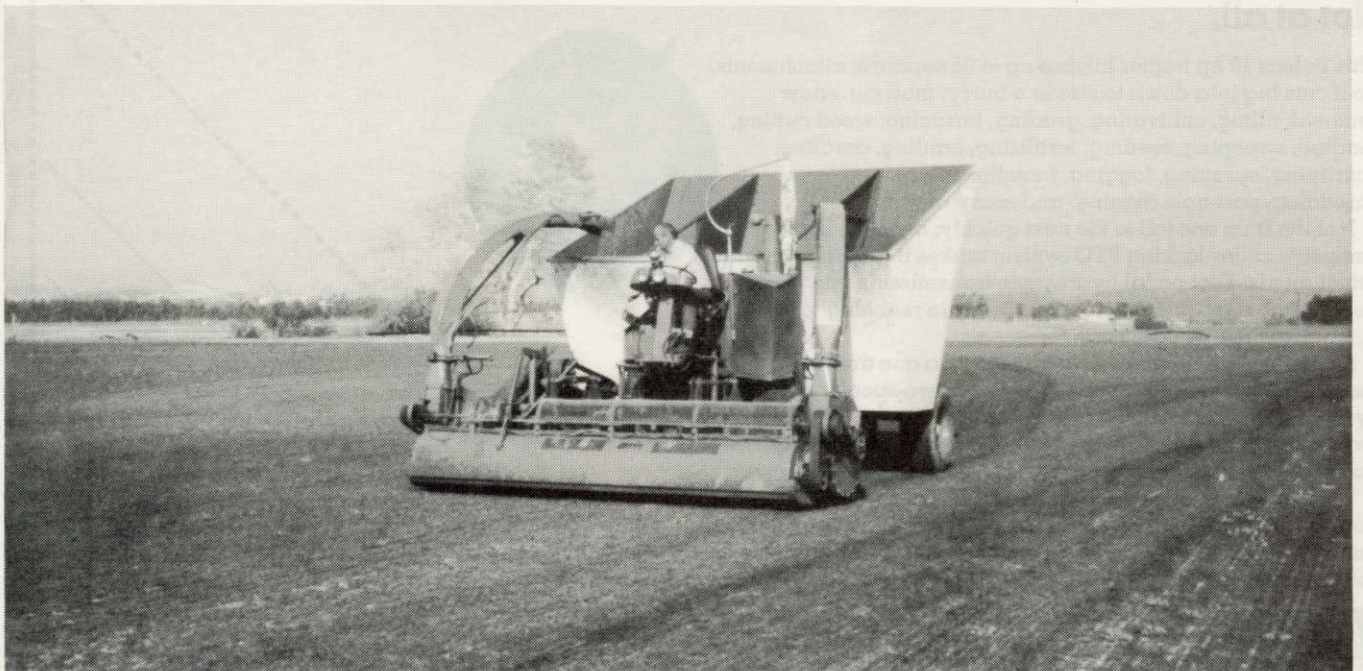
Custom built 12-foot flail mower is used in grass clipping program at Cal-Turf. Clippings are processed within 45 minutes of cutting.
