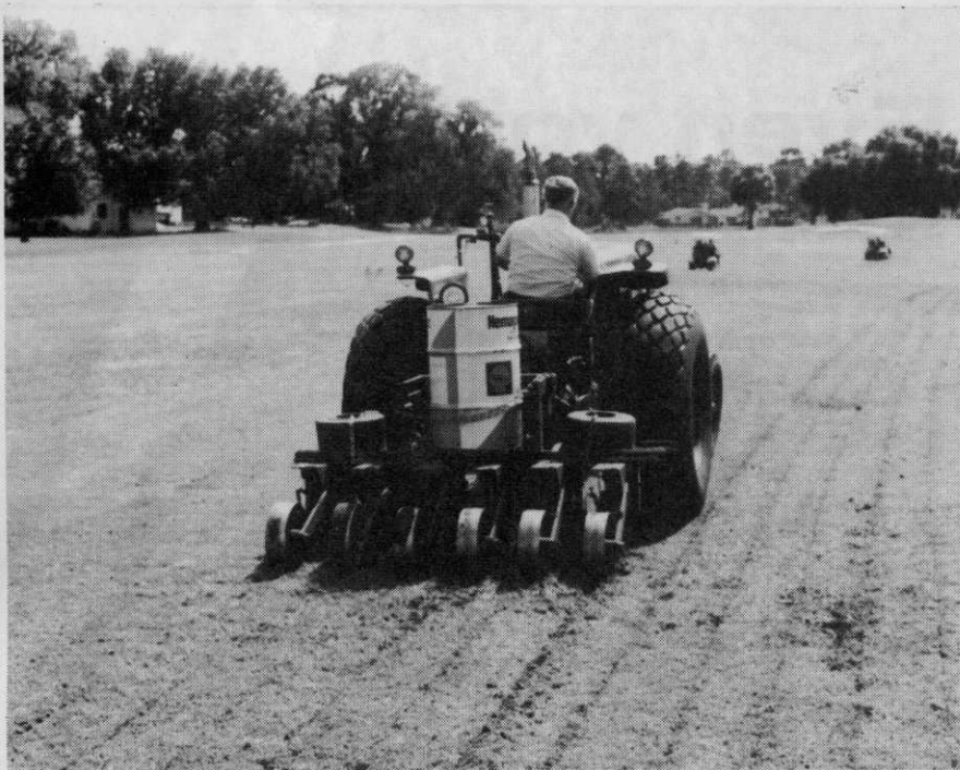
A rear view of the injection rig crossing a fairway. Tractor speed is set at six miles per hour. Note the cuts made by the machine.
