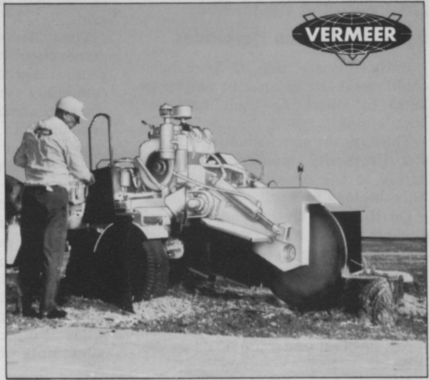
... and it's easy to maneuver! Digs 24" below the ground, up to 72" wide. Straight across cutting movement gives strict control next to streets, curbs, sidewalks, etc. Low silhouette design lets you operate easily in tight spots, under low objects.
